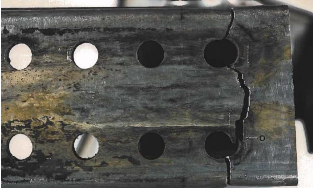
Figure 4. Example of Cracks Intersecting Outboard Bolt Holes; O indicates crack origin PA-28-181, 11,600 hours TIS
