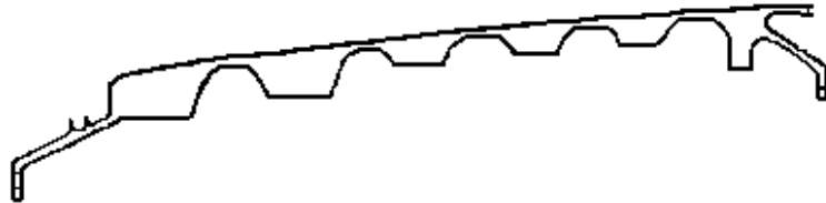
4.a - Ring Disk Drum Rotor Cross Section
