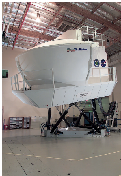
Symulator Boeinga B747-400 w centrum badawczym NASA Ames Research Center. Źródło https://www.aviation-systemsdivision.arc.nasa.gov/multimedia/cvsrf/images/747_ext_hi.jpg
